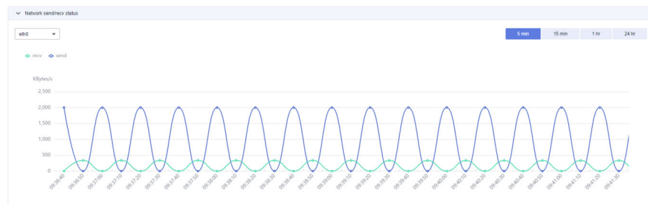
Figure 11-58 Network sending and receiving status
